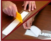
**PLACE MASK** over the graphic, making sure to smooth out any air bubbles.
