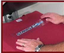
**PREHEAT & POSITION**— Preheat garment for 10 seconds, prior to application. Position & place cover sheet over graphic.
