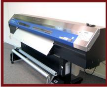
**FEED MATERIAL** into plotter/cutter so that the media faces up.
